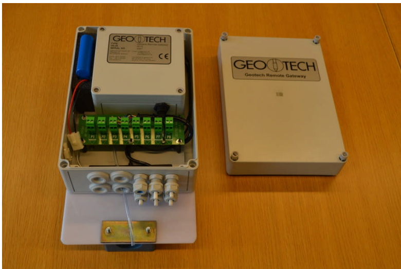
Fig. 3 – PVT Remote Gateway comprising small box with electronics, battery, antenna and terminal block.
